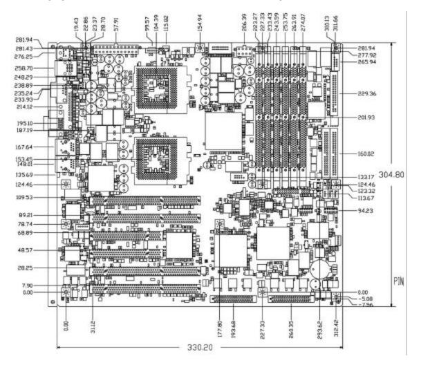
Figure 15. SDS2 Server Board Mechanical Drawing
